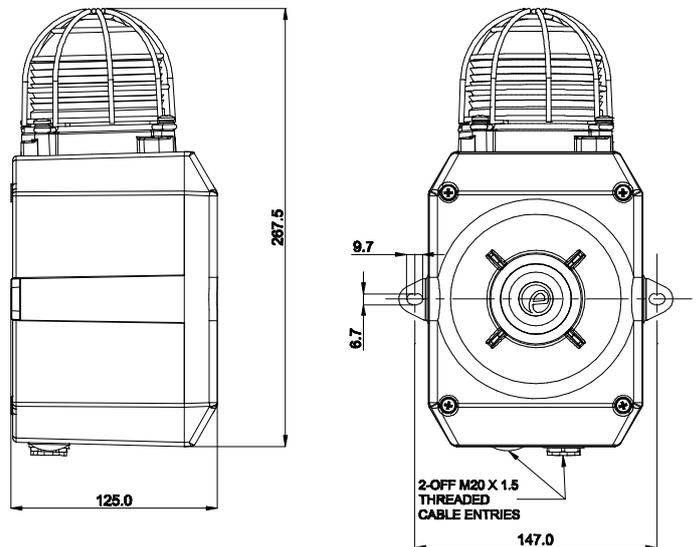
Always de-energize unit before removing cover. The installation of the units must be in accordance with any local codes that may apply and should only be carried out by a competent trained electrical engineer. The power terminals on the control unit are clearly marked and will accept up to 1.5mm<sup>2</sup> cable.
