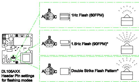
The LED beacon is set as standard to the 2Hz flash mode but it can be set to a steady on mode also. To alter the settings, change the position of the header pin as shown.
