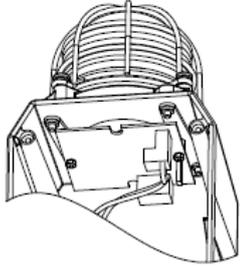
The xenon beacon is set as standard to 1Hz flash rate mode but it can be set to either 1.5Hz flash rate or double Strike flash pattern modes also. To alter the settings, change the position of the header pin as shown:
